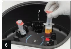
Centrifuge at 1500 rpm for five minutes (program A). Then carefully remove the double syringe.
