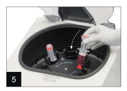
Place the syringe in the centrifugation container. Place a suitable counterweight (e.g., an ACP double syringe filled with water) on the opposite side.
